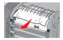
**c** If the jammed paper is not visible, then remove the fuser unit:
