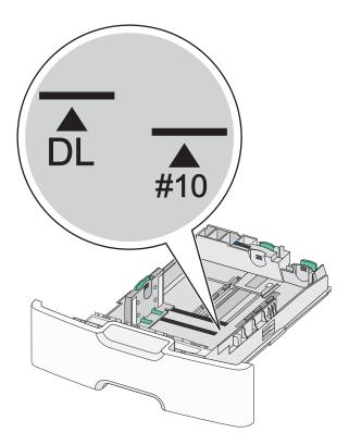
**4** Squeeze and slide the secondary length guide to the correct position for the paper size you are loading.
