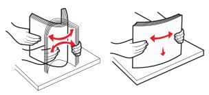
**5** Load the paper stack toward the back of the tray with the recommended printable side faceup.
