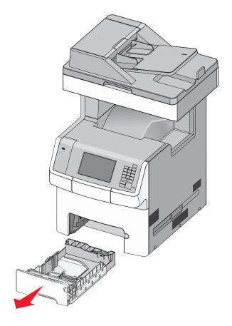
2 Squeeze and slide the width guide to the correct position for the paper size you are loading.
