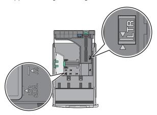
**3** Squeeze and slide the length guide to the correct position for the paper size you are loading.
