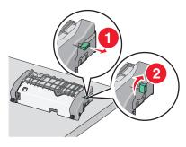
$\boldsymbol{f}$  Press the green arrow tab to the left, and then lift the top paper guide.
