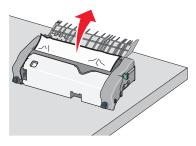
**h** Close the top paper guide. Make sure both sides of the paper guide are firmly seated.
