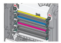
**2** Using the handholds on each side, lift and pull the fuser out of the printer.
