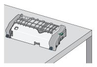
**e** Pull and then rotate the green rectangular knob clockwise to unlock the top paper guide.
