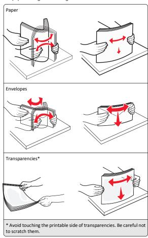
**4** Load the paper or specialty media. Slide the stack into the multipurpose feeder until it comes to a stop.
