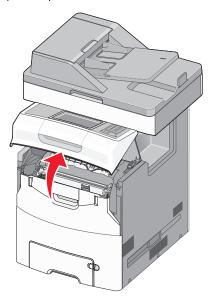
Warning—Potential Damage: To avoid overexposing the photoconductors, do not leave the front door open for more than 10 minutes.
