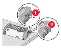
**f** Press the green arrow tab to the left, and then lift the top paper guide.
