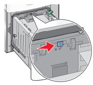
4 Push the length guide release latch to raise the length guide. Slide the guide to the correct position for the paper size you are loading, and then lock the guide.
