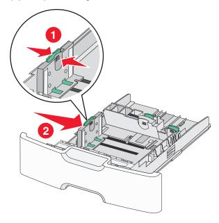
**Note:** Use the paper size indicators at the bottom of the tray to help position the width guide.
