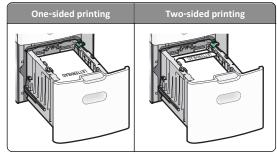
• Make sure paper does not exceed the maximum paper fill indicator located on the side of the tray.
