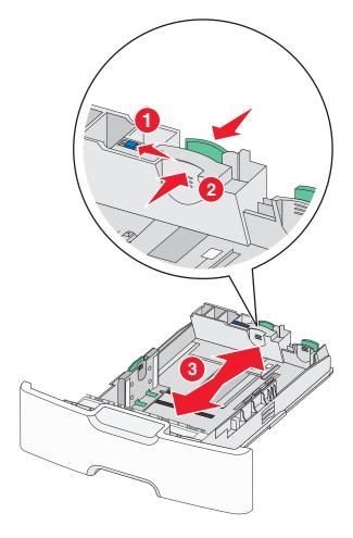
**3** Squeeze and slide the width guide to the correct position for the paper size you are loading.
