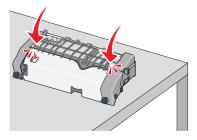
i Pull and then rotate the green rectangular knob counterclockwise to firmly secure the top paper guide.
