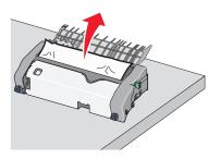
**h** Close the top paper guide. Make sure both sides of the paper guide are firmly seated.
