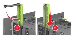
**d** Squeeze, and then slide the length guide to the correct position for the paper size you are loading.
