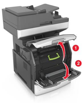
**2** Lift the green handle, and then pull out the toner cartridge from the printer.
