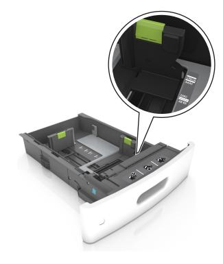
**3** Unlock the length guide, and then squeeze and slide the guide to the correct position for the size of the paper you are loading.
