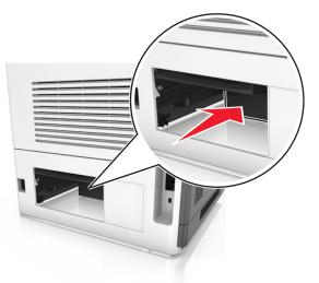
**5** Press down the rear duplex flap, then firmly grasp the jammed paper, and then gently pull the paper out.
