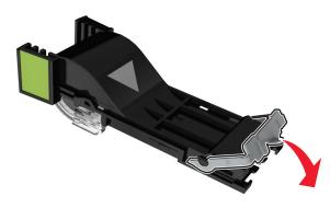
**5** Insert stapler cartridge back into the finisher until it *clicks* into place.
