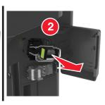
**3** Lift the staple guard, and then remove any jammed or loose staples.
