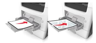
**Note:** When loading A6-size paper, make sure the multipurpose feeder extender rests lightly against the edge of the paper so that the last few sheets of paper remain in place.
