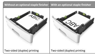
Make sure the paper is below the maximum paper fill indicator located on the side of the width guide. Overfilling may cause paper jams.
