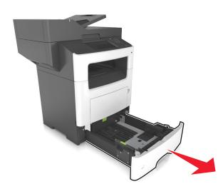
**2** Squeeze, and then slide the width guide tab to the correct position for the size of the paper you are loading.
